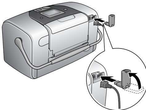
2. The Adapter's light comes on for one second. If the LED does not turn on, disconnect the Adapter from the printer, then reconnect it.
