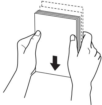
4. Load the paper with the printable side up so it is against the right edge guide, and slide it into the paper feeder. Then slide the left edge guide against the left edge of the paper. Make sure that the paper stack is loaded under the tabs inside the edge guides. You can load paper up to 20 sheets.
