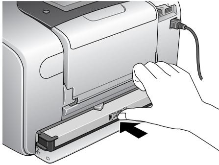
8. Slide the cartridge lock lever all the way to the right, then up slightly so that it catches.
