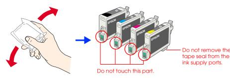
Install the ink cartridges as shown below. 3.
