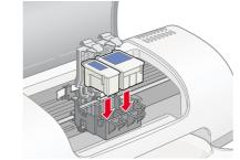
Install both ink cartridges. The printer will not work with only one
