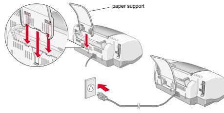
If the printer comes on when you plug in the power cord, turn off the printer by pressing down the O power button until the printer lights
