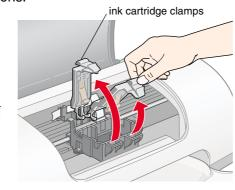
Do not move the print head by hand, as this may damage the printer.
