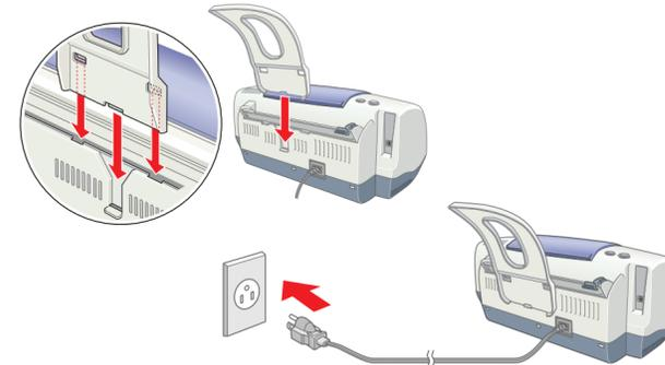
**Caution:** If the printer comes on when you plug in the power cord, turn off the printer by holding down the power button until light goes out.
