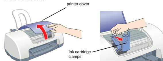
**Caution:** Do not move the print head by hand, as this may damage the printer.
