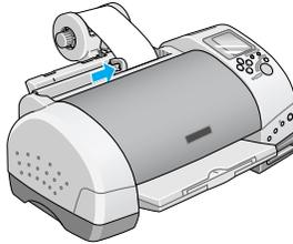
7. To load the paper correctly, you must hold the paper in place with your hand while you press the
