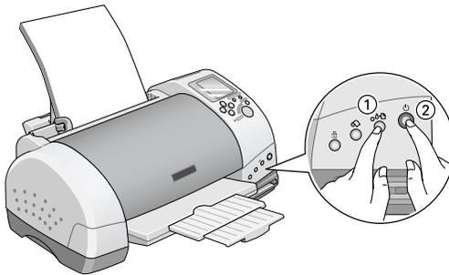
4. Release only the
