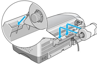
6. Gently insert the end of the paper into the printers as far as it will go, flush with the right edge guide. Slide the left edge guide against the left edge of the printer.
