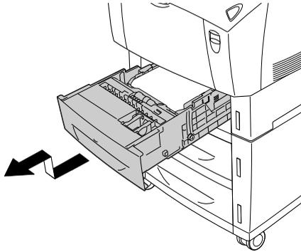
5. Remove the two screws securing the front of the unit to the printer.
