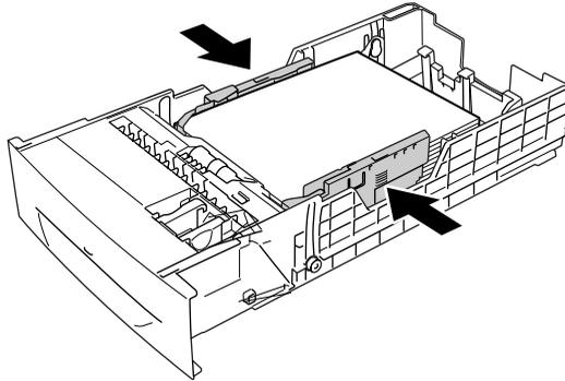
6. Insert the paper cassette gently into the printer, and push it back to the printer.
