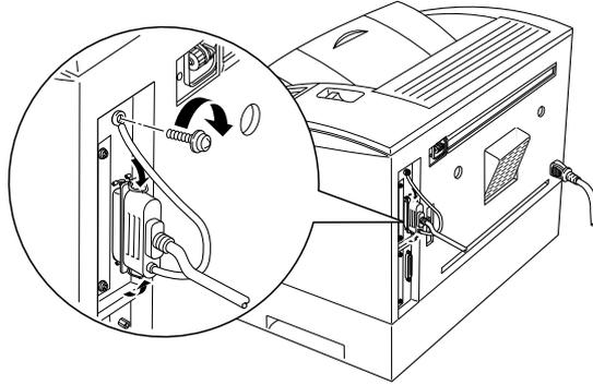
4. Connect the other end of the cable to your computer, and fasten it as required.
