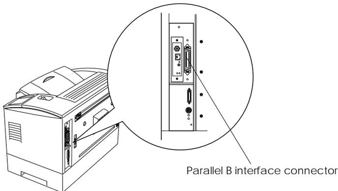
3. Secure the connector by squeezing the wire clips together until they lock in place on both sides of the connector.
