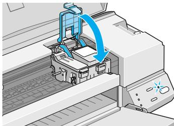
The illustration shows color ink cartridge replacement. To replace the black ink cartridge, lift up only the smaller clamp on the left.
