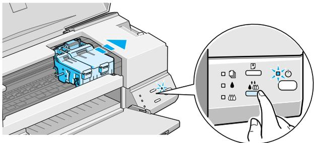
The printer starts cleaning the print head and the ⏻ power light begins flashing. Print head cleaning takes about one minute to complete.
