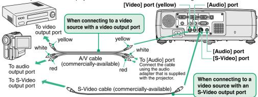
\* To play sound through the projector's built-in speaker, use the audio adapter (supplied with the projector) to connect an A/V cable (commercially available) to the [Audio] input port corresponding to the connected video source.
