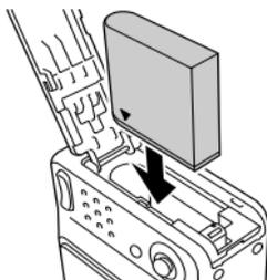
Installing the Li-ion battery
