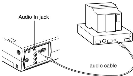
2. Connect the other end of the audio cable to the speaker or audio out port on the computer's sound card.
