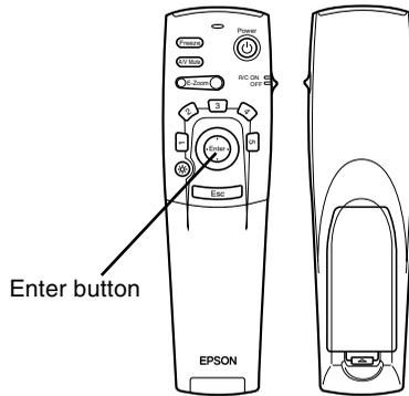
3. Press the Enter button to display a submenu.
