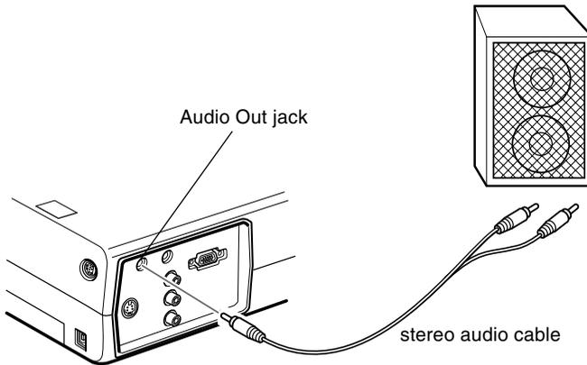
3. Connect the RCA plugs to the external amplified speaker or PA system. Insert the cable's red plug into the Audio R jack, and the white plug into the Audio L jack.
