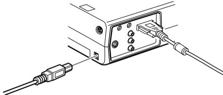
2. Connect the other end of the USB mouse cable to the mouse port on the back of the PowerBook.
