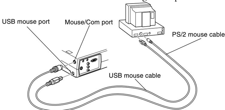
1. Connect the 9-pin end of the PS/2 mouse cable or, the USB mouse cable to the Mouse/Com or USB mouse port on the projector.
