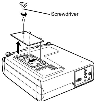
3. Loosen two mounting screws for the lamp with the same screwdriver, and pull out the lamp using the handle.
