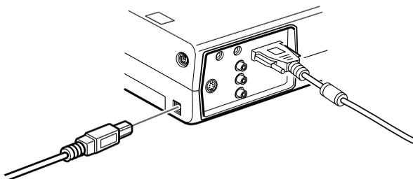
2. Disconnect your Macintosh's mouse cable. Connect the other end of the projector's USB mouse cable to the mouse port on your Macintosh.
