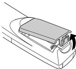
6. Insert the two alkaline dry cells LR6 (AA) included with the projector. Make sure the polarity of the batteries is correct.
