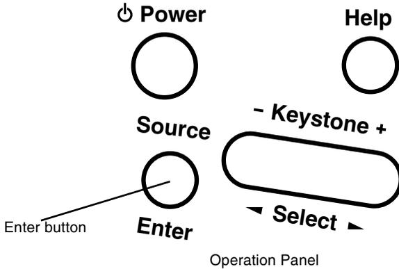
You can use the operation panel to control the projector instead of the remote control. However, you can program and access the custom features only using the remote control.
