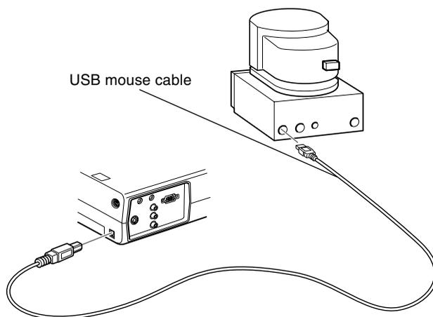
1. Connect one end of the projector's USB mouse cable to the USB Mouse port on the projector
