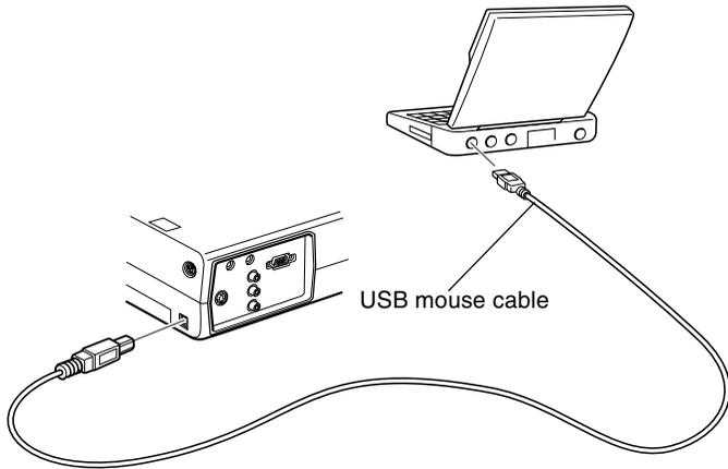
1. Connect one end of the projector's USB mouse cable to the USB Mouse port on the projector.
