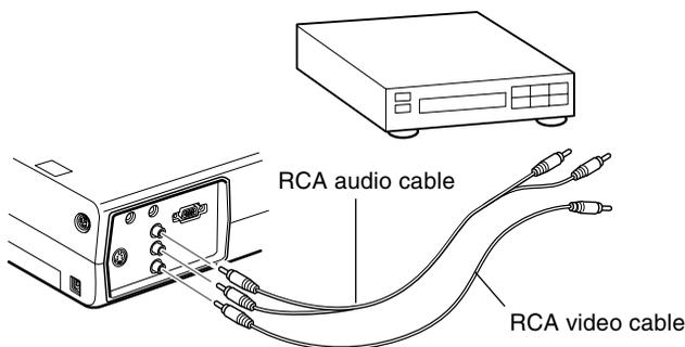
4. Connect the RCA audio cable to the Audio jacks of the projector: insert the white plug into the L jack and the red plug into the R jack. Connect the plug at the other end of the RCA audio cable to the audio output jacks of the video source.
