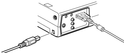
2. Disconnect your mouse from the mouse port on the back of your computer and replace it with the other end of the PS/2 mouse cable or USB mouse cable. (Your computer's mouse will be disabled while you are using the remote control as a mouse.)
