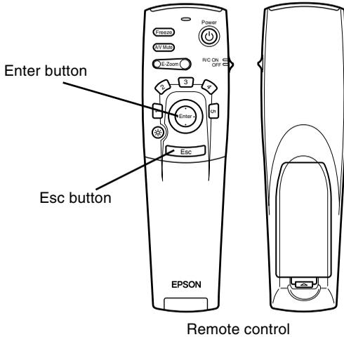
To use the remote control, point it towards the remote control receivers located at the front of the projector.
