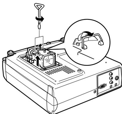
4. Mount new lamp. Check that the lamp orientation is correct, and then press it into place securely. Tighten the mounting screws for the lamp with the screwdriver.
