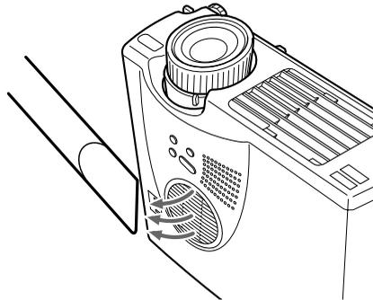
3. Use a small vacuum cleaner designed for computers and other office equipment to clean the filter.
