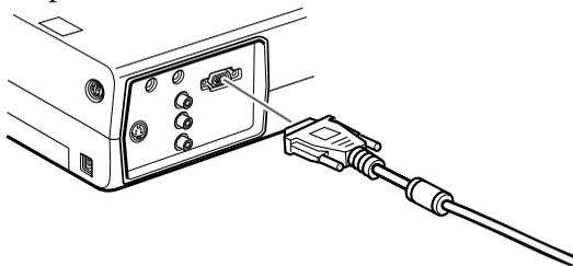
3. Connect the other end of the computer cable to the computer's video port.
