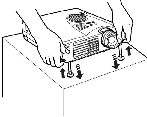
1. Stand behind the projector and support the front of it while you lift the foot adjust levers above the feet. This unlocks the feet so they can move up and down freely. Do not let the projector drop.
