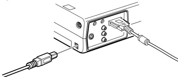
2. Connect the 6-pin (mini-DIN) end of the PS/2 mouse cable or USB mouse cable to the external mouse port or USB port on your laptop.
