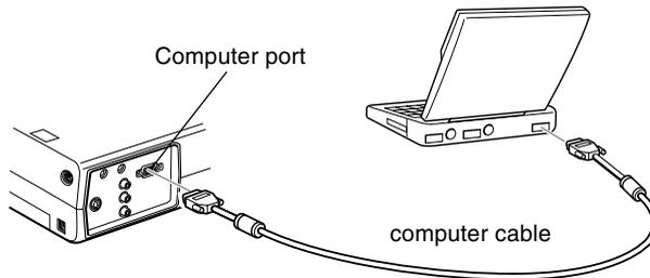
1. Connect one end of the computer cable to the projector's Computer port.
