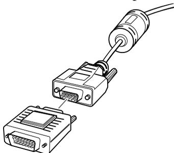
4. Connect the computer cable (with the Macintosh desktop adapter attached) to the video-out port on your Macintosh.
