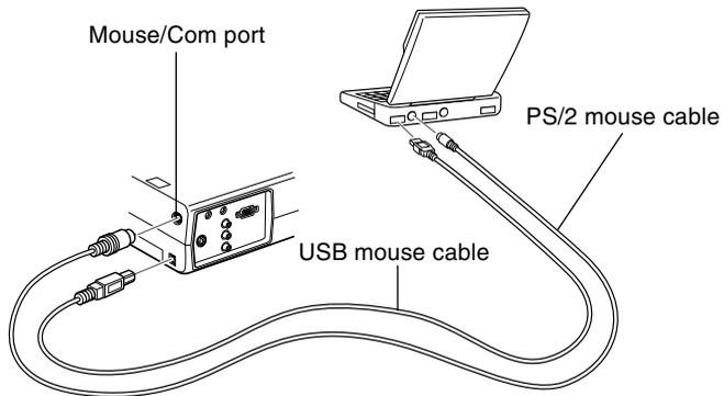
1. Connect the 9-pin end of the PS/2 mouse cable or USB mouse cable to the Mouse/Com or USB Mouse port on the projector.
