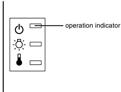
When the projector has cooled down, the operation indicator stops flashing and remains orange.
