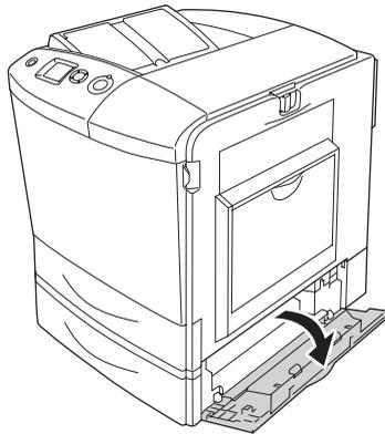
7. Gently pull out any sheets of paper that have fed part way into the printer.
