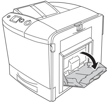
3. Push the latch on cover A to the left and open the cover.
