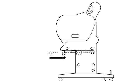
3. Likewise, fully insert and attach the long basket hooks to the lower guides.
