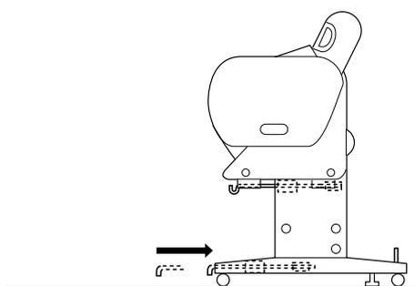
4. Turning the stitch side downward, spread the paper basket on the floor.
