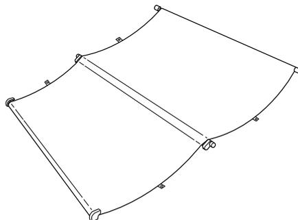
5. Holding the rear side shaft, pass it under the horizontal struts and insert the both joint sockets (H) on the stanchion pins.
