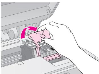
Squeeze the tab at the back of the empty/low cartridge and lift it straight out. Dispose of it carefully. Do not take the used cartridge apart or try to refill it.
