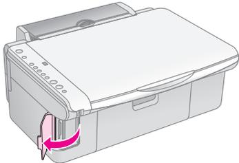
3. Make sure the memory card light is off and no cards are in any of the slots. Then insert your card into the correct slot. (➔ Page 9 for details.)
