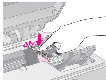
8. Replace any other cartridges that need to be replaced.
