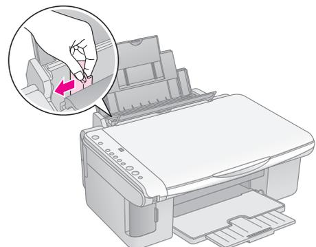
4. Insert the paper, printable side up, against the right side of the sheet feeder. Always load it short edge first, even for landscape printing.
