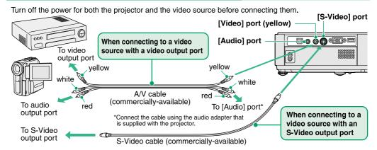
To play sound through the projector's built-in speaker, use the audio adapter (supplied with the projector) to connect an A/V cable (commercially available) to the [Audio] input port corresponding to the connected video source.
