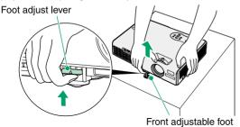
When the projector is tilted, automatic keystone correction operates. If you would like to make further minor adjustments to the result of automatic keystone correction, use \( \sigma \), \( \sigma \) on the projector's control panel.
