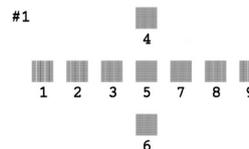
7. Look at the alignment pattern in each set and find the patch which is most evenly printed, with no noticeable streaks or lines.
