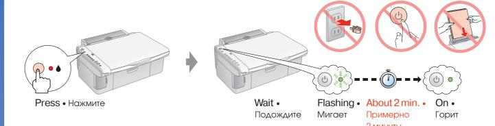
Note: The ink cartridges first installed in your EPSON STYLUS CX will be partly used to charge the print head. Subsequent ink cartridges will last for their full rated life.
