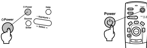
The Operation Indicator will change from blinking to being illuminated in orange once the cool-down process has been completed. The cool-down period will take approximately ninety seconds (depending on the surrounding temperature).
