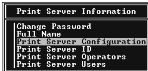
4. Select Printer Configuration from the Print Server Configuration Menu and press Enter.
