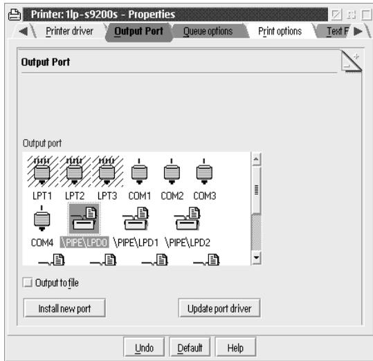
5. From the Output Port list box, select one from \PIPE\LPD0 to \PIPE\LPDn (where n is the maximum number of LPD ports). The \PIPE\LPD -Settings dialog box will appear.
