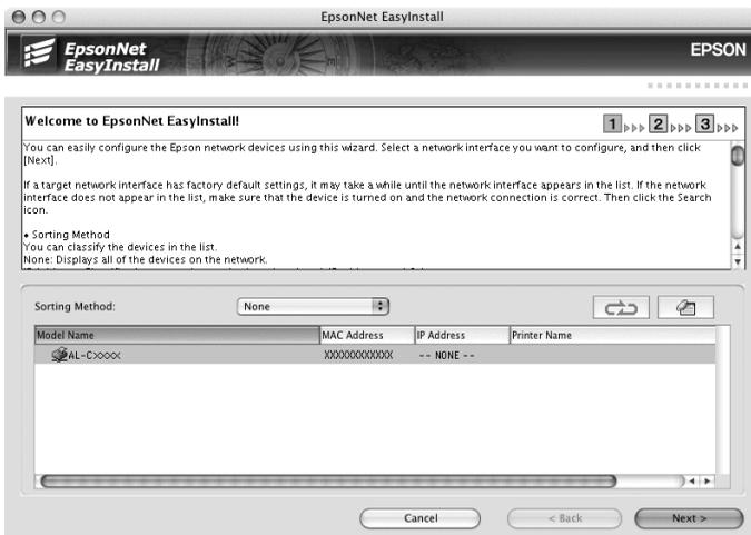
4. Select a method for specifying the IP address. If you select Automatic, DHCP becomes available and assigns an IP address automatically. If you want to set the IP address manually, select Manual and then enter the IP address, subnet mask, and default gateway. Click the Next button.
