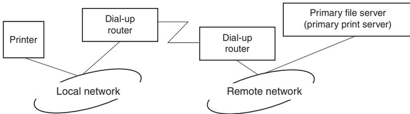
Depending on the router settings, the NetWare protocol can be used without a file server on a local network. This setup follows the same pattern as that described above.
