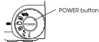
The lens extends from the camera when a red icon is selected with the dial switch and the camera is turned on. The lens retracts when you turn the camera off.
