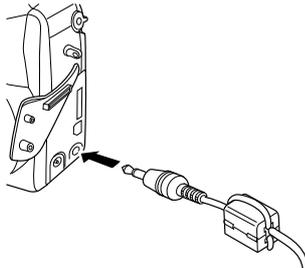
4. Connect the other end of the AV cable to the audio and video input ports on the television.
