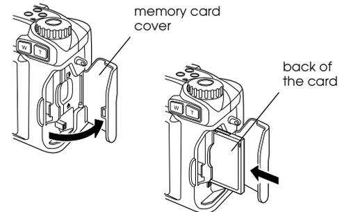
To remove the card, push in the eject button below the memory card slot. Then, remove the card and close the cover.
