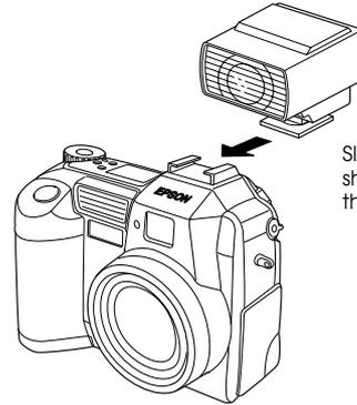
Slide the flash into the hot shoe and make sure that the connection is secure.
