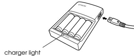
3. Plug the power cord into an electrical outlet. The red charger light turns on, indicating that the charger is working.
