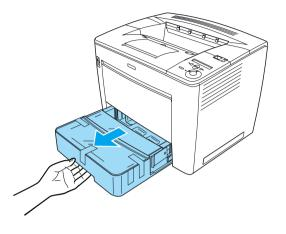
3. While pressing the gray stoppers located on both sides of the paper cassette, pull the cassette out from the printer.
