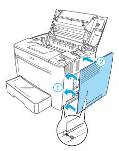
2. Fasten the right cover with screws, as shown below.
