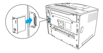
4. Secure the interface card with its screws.
