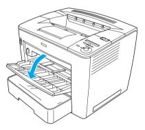
2. While squeezing the guide lock on the right side of the paper guide, slide the paper guide to accommodate the paper you are loading.
