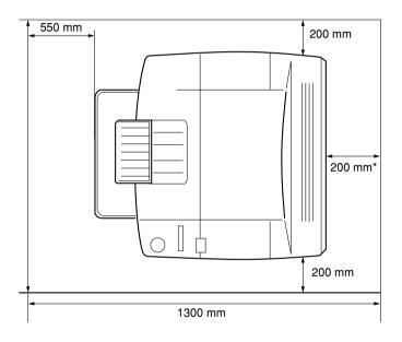
\* 300 mm when the optional Duplex Unit is installed, and 450 mm when the optional 4-Bin Mailbox is installed.
