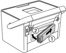
3. Attach the battery cover as shown below.
