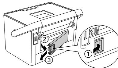
4. Insert the battery into the compartment in the direction shown below until it is fixed in place.
