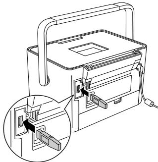
2. The Adapter's light comes on for one second. If the LED does not turn on, disconnect the Adapter from PictureMate, then reconnect it.
