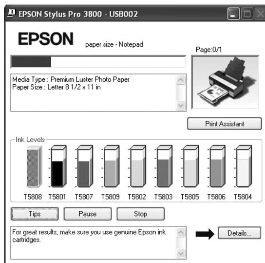
The Progress Meter indicates the progress of the current print job and provides printer status information when bi-directional communication between the printer and your computer is established. This meter also displays helpful tips for better printing and error messages.
