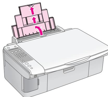
2. Open the output tray and slide out the extensions.
