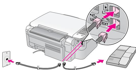
3. Connect the other end of the cable to the **EXT.** port on the back of the product.
