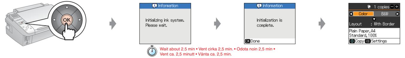
**Note:** The ink cartridges first installed in your printer will be partly used to charge the print head. These cartridges print fewer pages compared to subsequent ink cartridges.
