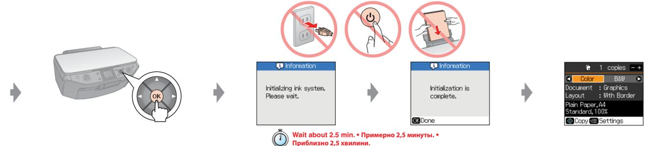
**Note:** The ink cartridges first installed in your printer will be partly used to charge the print head. These cartridges print fewer pages compared to subsequent ink cartridges.
