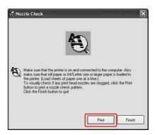
Check if there are missing dots on the nozzle check pattern.
