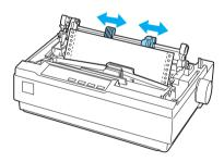
7. Make sure your paper has a clean, straight leading edge. Open the sprocket covers. Fit the first holes of the paper over the sprocket pins and then close the sprocket covers. Slide the right sprocket unit to remove any slack in the paper and then lock it in place.
