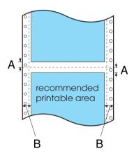
A The minimum top and bottom margins above and below the perforation are 4.2 mm (0.17 inch) each.
