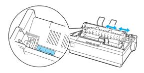
4. Make sure your paper has a clean, straight leading edge. Open the sprocket covers. Fit the first holes of the paper over the sprocket pins and then close the sprocket covers. Slide the right sprocket unit to remove any slack in the paper and lock it in place. Now the paper is in the paper-park position.
