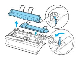
2. Squeeze the tractor's lock tabs gently on both sides, and then rotate the tractor up to pull it away from the printer.
