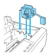
3. Insert the motor unit plug into the connector on the printer.
