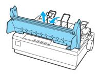
3. Make sure that the print head is in the middle of the printer. (If it is not, turn on the printer, and then, turn off the printer.) Then remove the ribbon cartridge from the printer.
