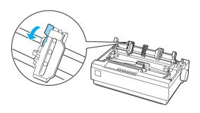
5. Insert the paper into the bottom paper slot or into the rear paper slot as shown below, and pull it up. Position the paper using the scale on the printer as a guide. The printer prints to the right of the position marked 0.
