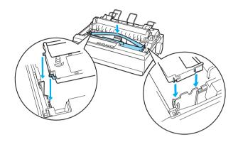
7. Use a pointed object, such as a ball point pen, to guide the ribbon between the print head and ribbon guide.
