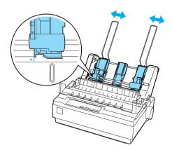
6. Pull the paper set levers all the way forward until the paper guides retract and lock open to allow for paper loading.
