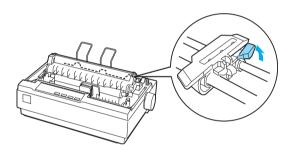
3. Slide the left sprocket unit using the scale on the printer as a guide. The printer prints to the right of the position marked 0. Push the sprocket lock lever back to lock it in place. Then slide the right sprocket unit to match the width of your paper, but do not lock it. Move the paper support so it is midway between the sprocket units.
