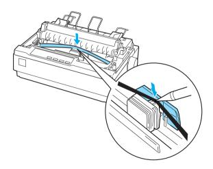
8. Turn the ribbon-tightening knob in the direction of the arrow to help feed the ribbon into place; it should not be twisted or creased.
