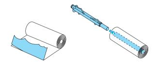
5. Set the shaft and paper roll onto the roll paper holder. Orient the roll so that paper feeds from the bottom of the roll. Then turn on the printer.
