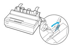
2. Slide the left edge guide until it locks in place at the guide mark. Next, adjust the right edge guide to match the width of your paper.
