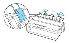
3. Slide a sheet of paper down firmly between the edge guides until it meets resistance.
