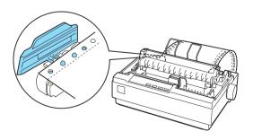
5. To separate the incoming paper from the printed paper, attach the paper guide by holding it horizontally and fitting its notches over the printer's mounting posts as shown below. Then slide the paper guide toward the front of the printer until you feel it click and adjust the edge guides to the width of the paper.
