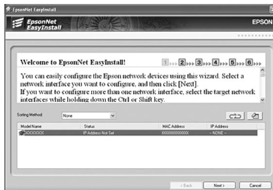
8. Select a method for specifying the IP address. If you select **Automatic**, DHCP becomes available and assigns an IP address automatically. If you want to set the IP address manually, select **Manual** and then enter the IP address, subnet mask, and default gateway. Click the **Next** button.
