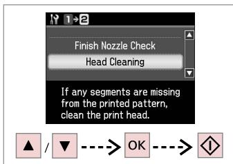
Izberite **Head Cleaning** in začnite.
