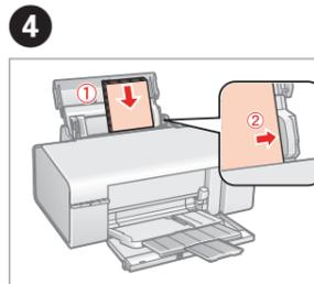
Load the paper with the printable side up.
