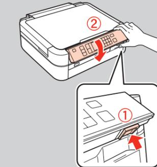
Installing the Ink Cartridges
