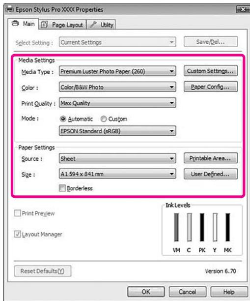
Set Media Type, Source, Size (Roll Width if roll paper is loaded), and so on.
