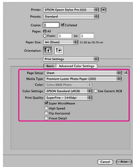
Select the same media type that you loaded in the printer. Normally, you can print correctly just by making the settings in the Print Settings dialog.
