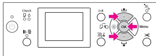
The Power light starts flashing and the head cleaning starts (it takes 2 to 9 minutes.) The cleaning is finished when the Power light is on.
