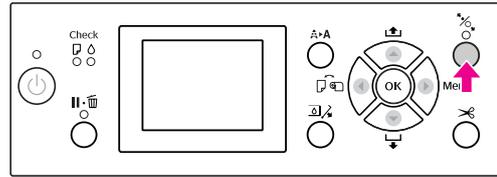
After a few seconds, the paper moves to the printing position. When you press the button, it moves immediately.
