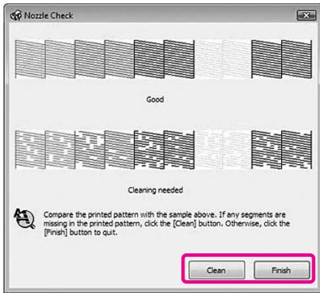
After printing a nozzle check pattern, make sure that the nozzle check pattern printing is complete before starting to print your data or cleaning the print head.
