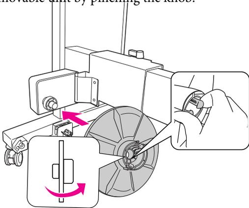
**Installing a take-up reel core**
