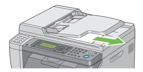
4. Remove any paper in the center output tray if there is. Close the output tray extension if it is extended.
