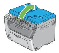
8. Remove the document from the ADF feed roller or the feed area by carefully pulling the document in the direction of the arrow shown in the following illustration.
