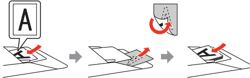
Do not load paper above the line just under the ▼ arrow mark on the ADF.
