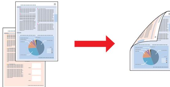
Choose automatic or manual printing. When you print manually, the even-numbered pages are printed first. Once these pages are printed, you can reload them to print the odd-numbered pages onto the opposite side of the paper.
