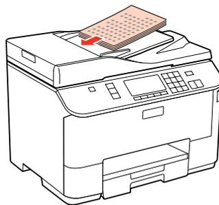
**4** Slide the edge guide until it is flush with the originals.
