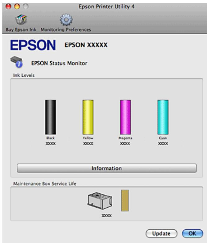
When ink is low/expended or the maintenance box is nearly full/full, a **How to** button appears. Click **How to**, and EPSON Status Monitor will lead you step by step through the ink cartridge or maintenance box replacement procedure.
