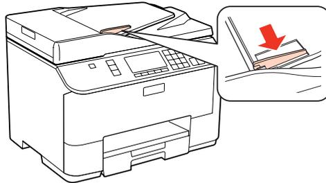
**3** Insert the originals face-up and short edge first into the Automatic Document Feeder.
