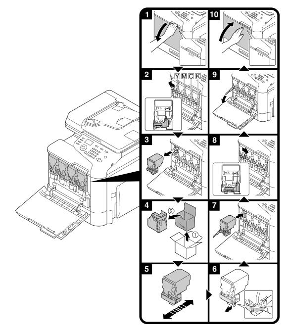
The procedure for replacing toner cartridge is the same for all toner colors. As an example, the procedure for replacing the yellow toner cartridge is described.
