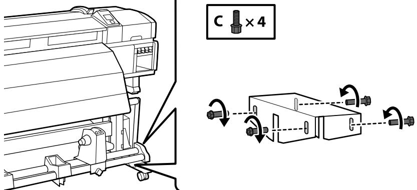
Keep the four screws in the figure on the left provisionally tightened until parallel adjustment is completed.
