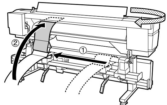
**[8]** At the front side of the printer, check the positions of the white line on the platen and the line you drew in step [6] while the adjustment paper is taut. If the line you drew is not aligned with the white line as shown in the figure on the right, go to step [9]. If the lines are aligned, go to step [10].
