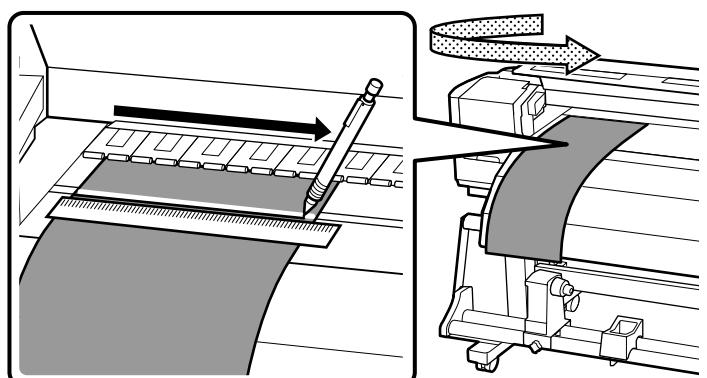
**[7]** Pull out the adjustment paper from the rear side, pull it to the left end of the roll core, insert it into the printer, and then feed it all inside.
