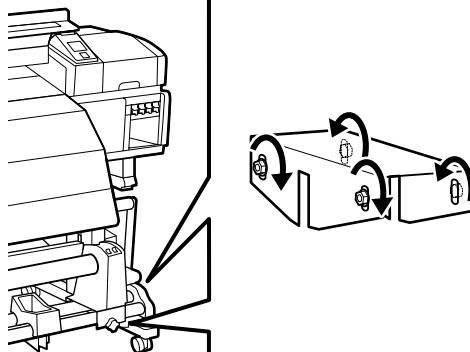
Fully tighten the four screws that you provisionally tightened.
