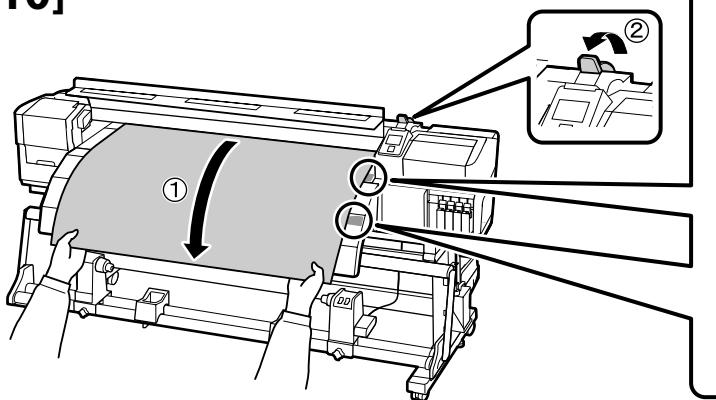
Pull out the media until the right end is paralleled with the scale marks on the two labels.
