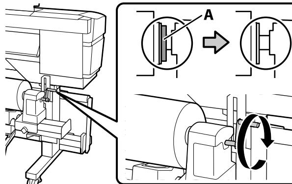
Turn the handle until part A in the upper left figure is hidden. Once part A is hidden, do not turn the handle any further.
