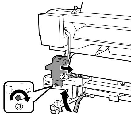
If the roll of media has the outer diameter which is less than 140 mm, lift it up by your hands, and set it to the roll holder.
