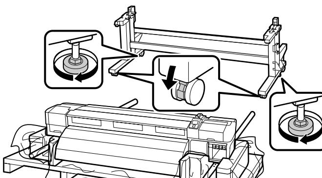
Before using the printer, be sure the stand is fixed in place. When moving the printer, rotate the adjusters in the opposite direction to raise them and then unlock the casters.
