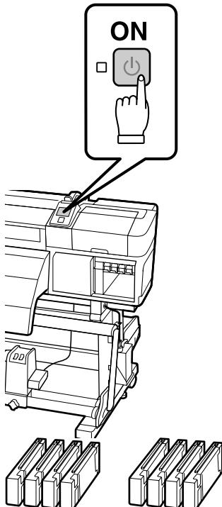
Turn on the power and configure the initial settings, such as the language and date. Then, follow the instructions on the control panel screen to perform the initial ink charging. In the initial ink charging, first wash the head (charge and discharge the cleaning liquid), and then charge the ink. After charging the cleaning liquid, remove the cleaning cartridge, discharge the cleaning liquid, and then install the ink cartridge.
