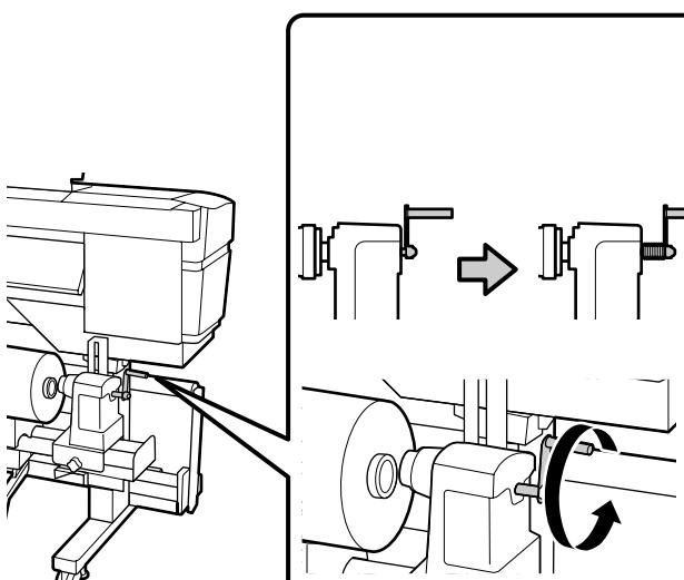
If the handle shaft of the right side roll holder is pressed in, turn it to the front until the handle can no longer be turned.
