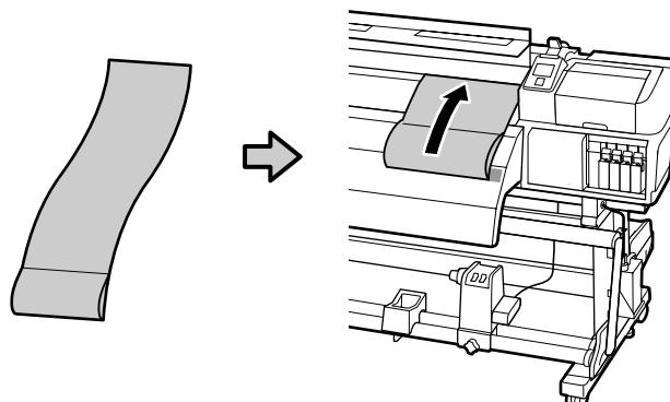
Position the rolled side of the adjustment paper at the bottom, and insert it into the printer from the top end.
