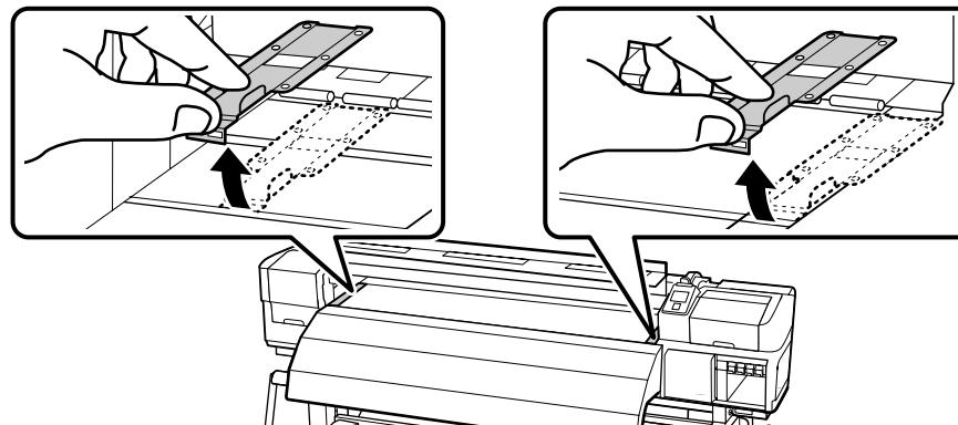
The removed media holding plate is used when printing on media with a thickness of less than 0.4 mm.
