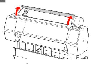
Press the <sup>\*</sup>/<sub>2</sub>, button to release the paper presser.
