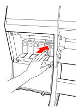
Carefully pull the expended cartridge straight 6 out of the slot.
