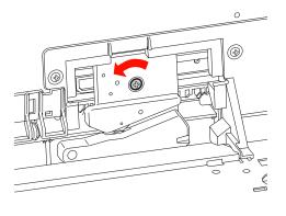
Carefully remove the old cutter from the printer.
