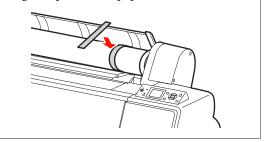
4 To unlock the adapter holder, push the lock lever of the adapter holder down firmly. Move the adapter holder to the left with the handle until the end. Then take it off from the holder axis.
