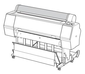
Load the sheet into the paper insertion slot until it meets resistance.
