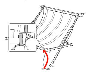
4 Turn the attachment part towards the printer and then fit it to the gutter of the basket guide by pressing down on the handle section.
