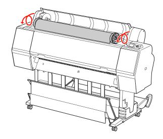
6 Pull up the lock lever of the adapter to unlock. Then remove the roll media adapter from the roll paper.
