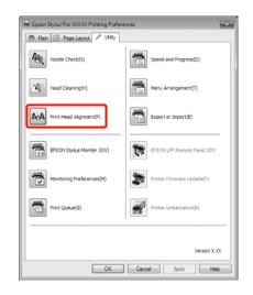
The sensor reads the adjustment pattern while it is printing, and automatically registers the optimum adjustment value to the printer.
