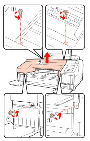
Remove when the optional SpectroProofer is installed.
