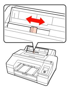
5 Insert the paper into the rear manual feeder with the printable side face up as shown in the illustration.
