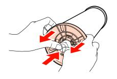
If the flange does not come off easily, lightly tap the end of the spindle on the black flange side.
