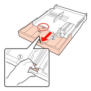
When extending the paper cassette, pull the lever in the paper cassette while extending. It locks in place when the lever is released.
