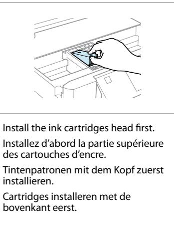
Install the ink cartridges head first.
