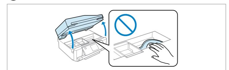
When instructed to install the cartridges, open the upper section.
