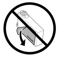
Do not remove the transparent seal from the bottom of the cartridge; otherwise, the cartridge may become unusable.
