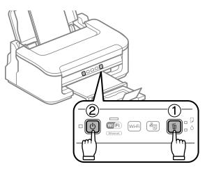
5 When the product turns on, release both the buttons. The product prints the nozzle check pattern.
