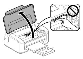
Make sure the ink cartridge holder is at the ink cartridge replacement position.
