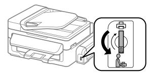
Make sure to install the cap onto the ink tank securely.
