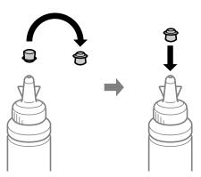
Install the cap onto the ink tank securely.
