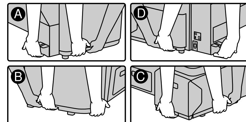
When lifting the printer unit, only hold the highlighted area. Otherwise, it may affect normal operation and printing.
