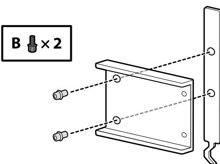
Give the screws shown in the figure a couple of turns to fasten the parts temporarily. The items in the following steps can not be attached if the screws are too tight.
