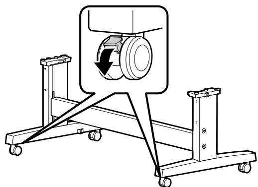
**!** Before using the printer, be sure the stand is fixed in place. When moving the printer, unlock the casters.
