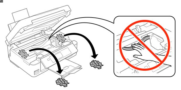
Close the scanner unit. If the jammed paper remains near the output tray, carefully remove the paper.
