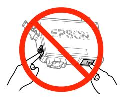
Do not leave the product with the ink cartridges removed or do not turn off the product during cartridge replacement. Otherwise, ink remaining in the print head nozzles will dry out and you may not be able to print.
