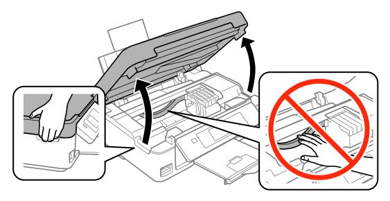
Make sure the ink cartridge holder is at the ink cartridge replacement position.
