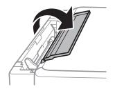
Slide out the paper support and the output tray and then raise the stopper.
