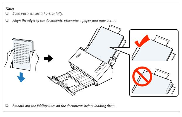
Slide the edge guides to fit the edge of the paper.
