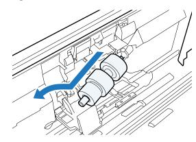
Remove the roller from the axis.
