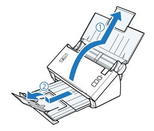
2 Slide the edge guides on the input tray all the way out.
