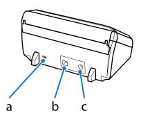
a. security slot b. USB interface connector c. DC inlet
