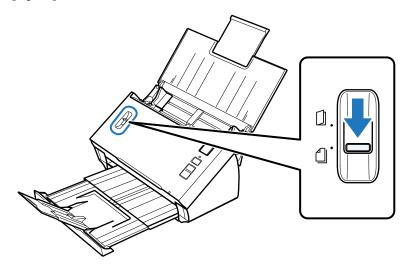
4 Load only the first page of your documents into the input tray with the printed side facing down and the top edge facing into the feeder.
