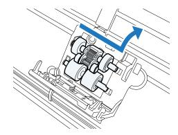
6 Attach the new lower pickup roller in the correct position.
