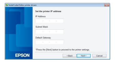
Once the next screen appears, disconnect the USB cable from the printer. Next, select the network connection method to be used and proceed with configuring the settings.
