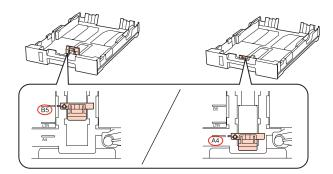
4 Load paper toward the edge guide with printable side face down, and check that the paper is not sticking out from the end of the cassette.
