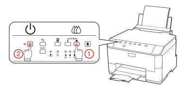
A test page prints showing a nozzle check pattern. If the pattern has gaps, you need to clean the print head.
