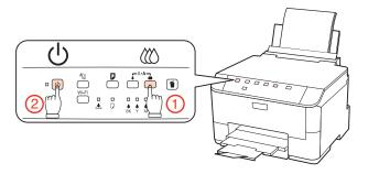
When the printer turns on, release both the buttons. The printer prints the nozzle check pattern.
