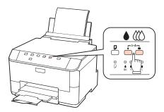
The printer starts cleaning the print head and the  $\mathcal{O}$  light begins flashing.
