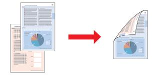
Choose automatic or manual printing. When you print manually, the even-numbered pages are printed first. Once these pages are printed, you can reload them to print the odd-numbered pages onto the opposite side of the paper.
