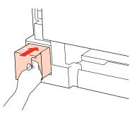
7 Push the button on either side of the rear unit at the same time, and then reattach the unit.
