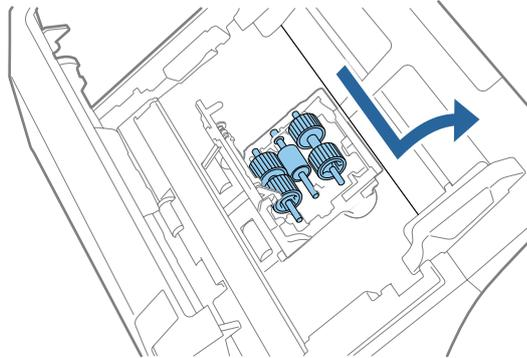
**6** Remove the upper pickup roller from the axis.
