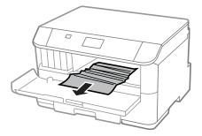
Close the front cover. If the jammed paper remains near the output tray, carefully remove the paper.
