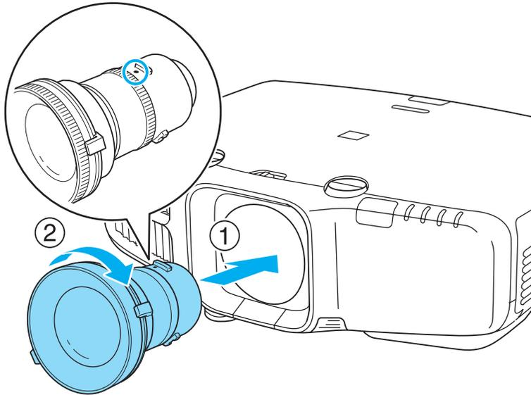
Turn the torque ring on the lens unit to adjust the torque for the zoom ring.
