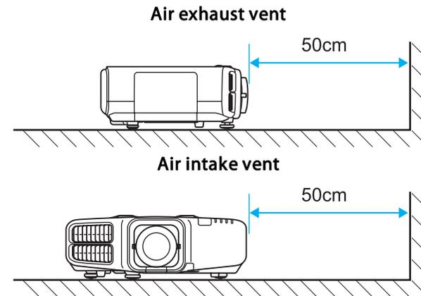
When setting up multiple projectors, make sure there is a gap of at least 50 cm between the projectors. Also, make sure the heat coming out of the air exhaust is not taken in through the air inlet.
