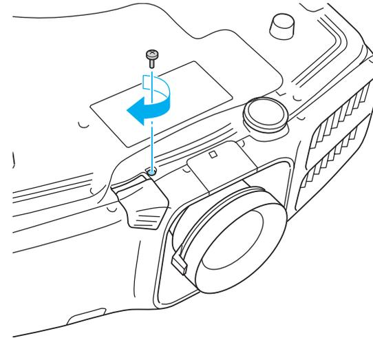
Make sure you fix the lens unit removal button with the screw to prevent the lens unit from being stolen.
